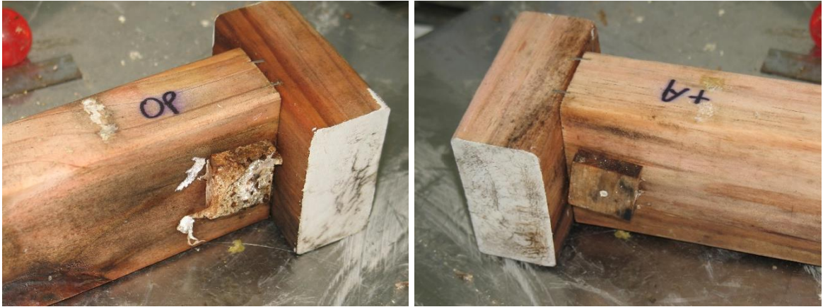
Figure 7: Established mould but no decay observed on boron treated radiata pine sample (sample 30).
