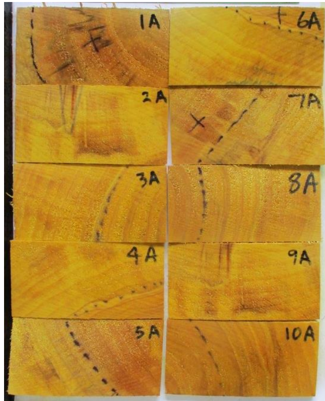
Figure 8: Heartwood\sapwood spot tests for Poplar boron treated 90 x 45 mm
