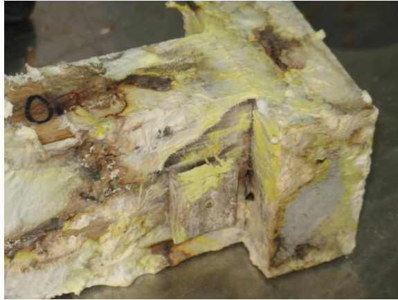
Figure 1: Untreated Poplar sample with extensive mycelium at the Op end (sample 13).
