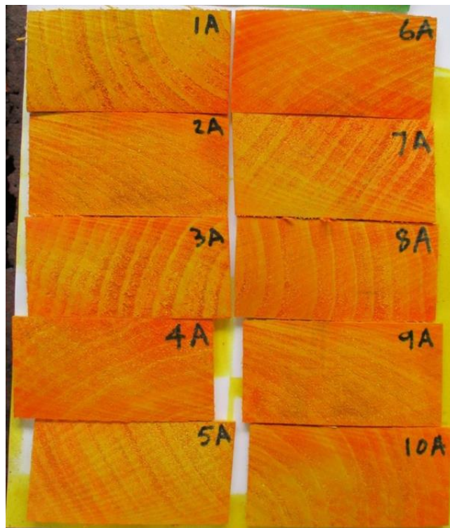
Figure 9: Penetration spot tests for Poplar boron treated 90 x 45 mm
