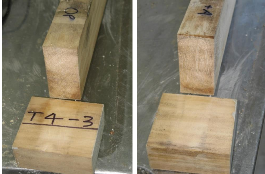
Figure 4: Boron treated Poplar sample without decay on the surface or in the joint at either end (sample 9).
