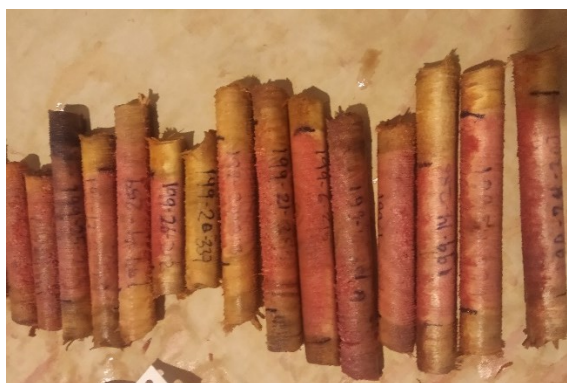
Figure 3: E. globoides cores with heartwood dyed pink after application of methyl orange.
