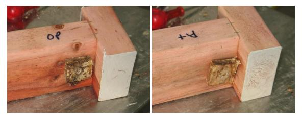
Figure 6: No decay or mycelium observed on boron treated radiata pine sample (sample 25).
