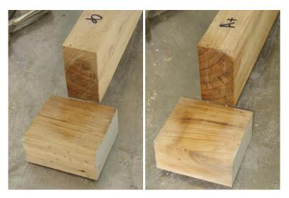
Figure 3: Boron treated Poplar sample without decay in the joint at both ends (sample 1).
