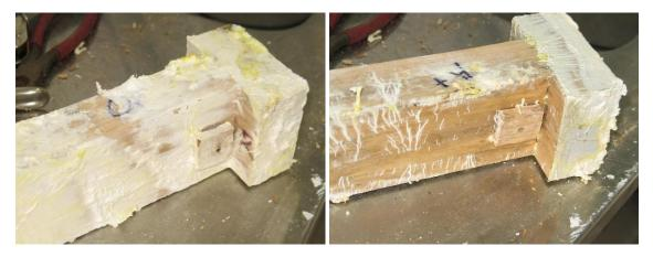
Figure 4: Severe mycelium on both ends of a sample of untreated radiata pine from Northland (sample 31).
