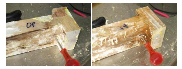
Figure 5: Established decay at the Op end, and severe decay at the Ax end a sample of untreated radiata pine from Northland (sample 38).
