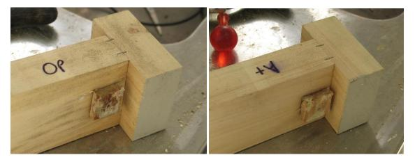
Figure 2: Boron treated Poplar sample with light mould and no mycelium at either feeder block (sample 6).
