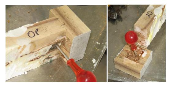
Figure 1: Untreated Poplar sample with established decay on the surface and in the joint at the Op end. (sample 19).
