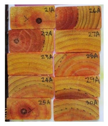
Figure 10: Heartwood\sapwood spot tests for radiata pine boron treated 90 x 45 mm
