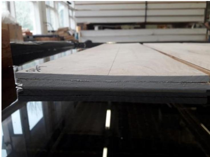
**Figure 7.** Delamination in an engineered oak board during water soaking
