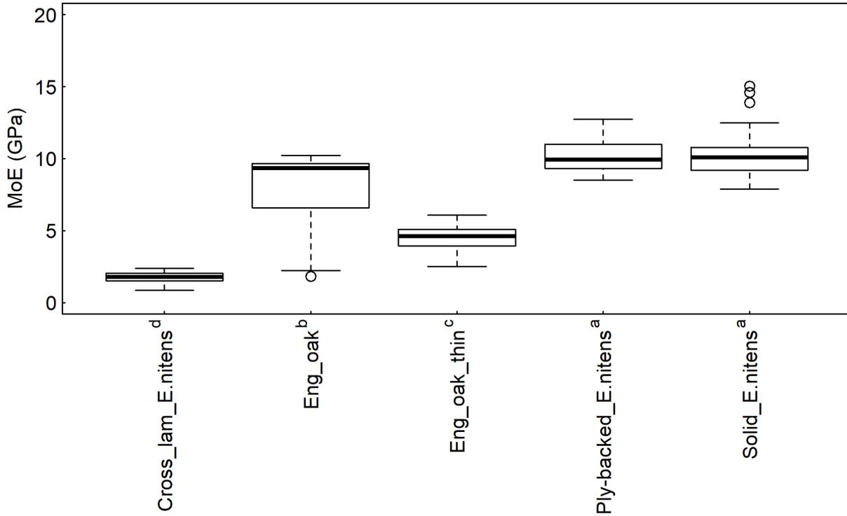
**Figure 9.** Modulus of elasticity (MOE) of different flooring types. Superscript letters indicate treatments that are not significantly different (95% confidence level).
