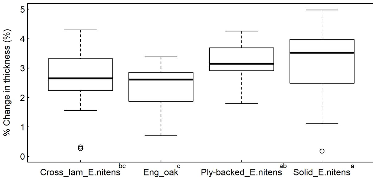
**Figure 2.** Change in thickness between 35 and 90% RH conditions for each board type. Superscript letters indicate groups that are not significantly different to each other (95% confidence level)
