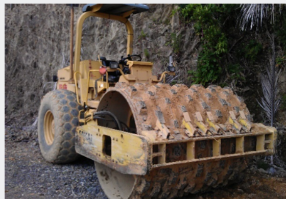
Pad foot roller suitable for compacting cohesive soils.
