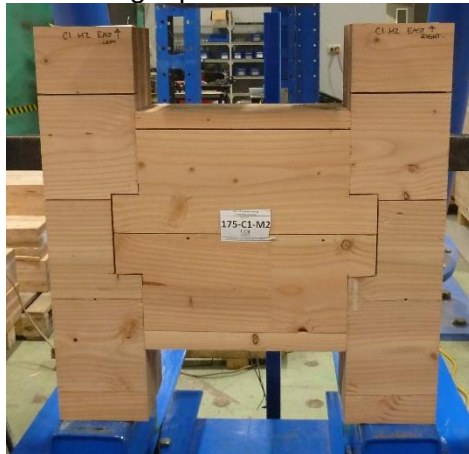
Figure 25: Load perpendicular to outer CLT layer
