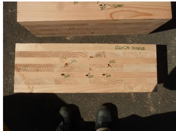
Figure 56: CLT7-375X - Timber embedment crushing
