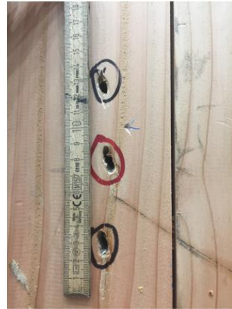
Figure 71: CLT crushing / embedment
