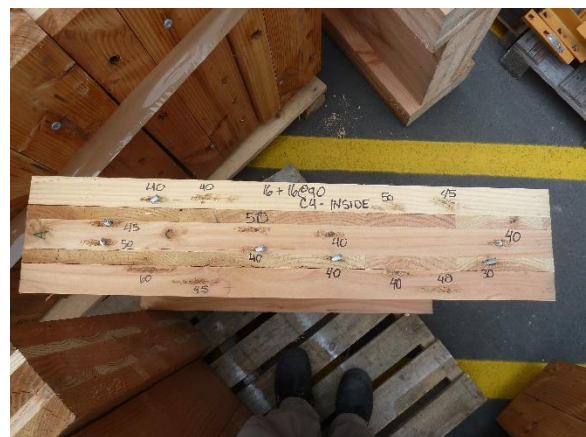
Figure 57: CLT5-16X+16 - Timber embedment crushing
