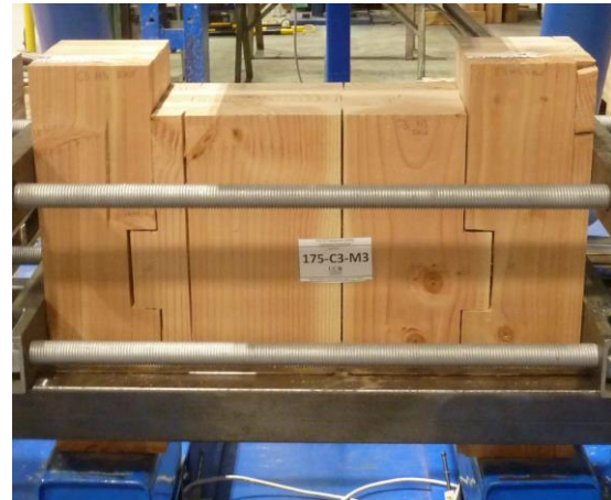
Figure 26: Load parallel to outer CLT layer
