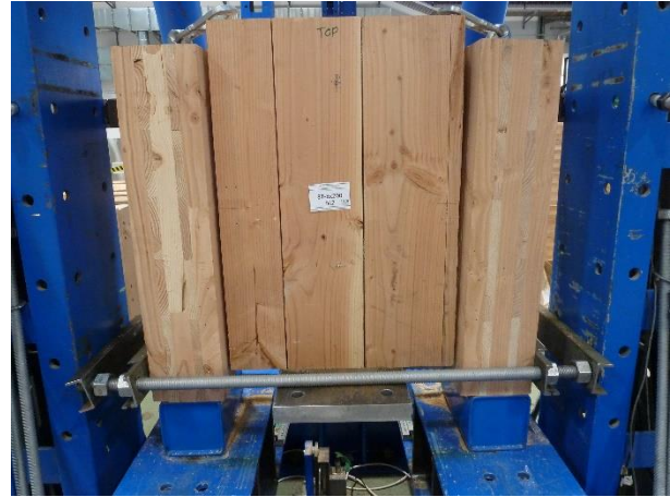
Figure 55: CLT5-8T test - 80mm displacement
