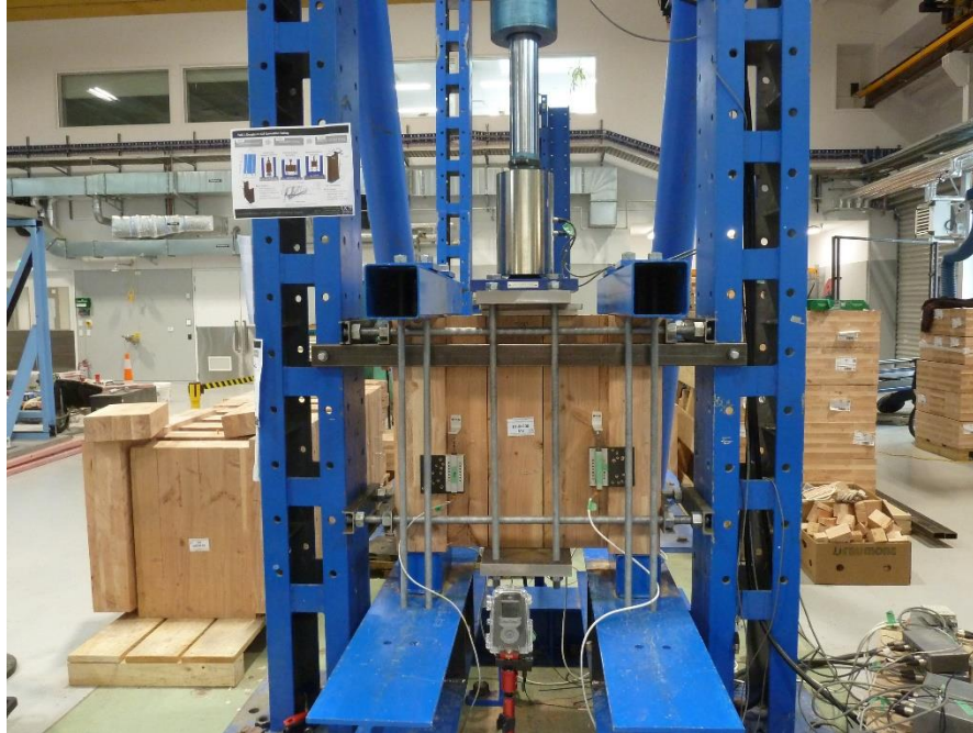
Figure 8: Screwed connection testing set-up
