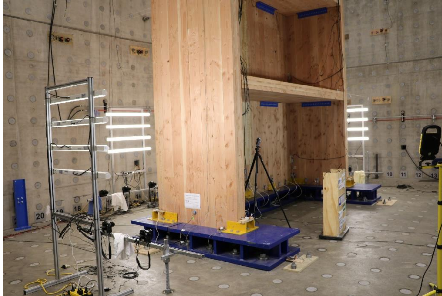
Figure 68: PTV set-up with cameras and lighting
