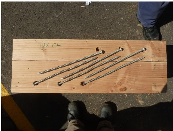
Figure 53: CLT7-375X - Screws post test
