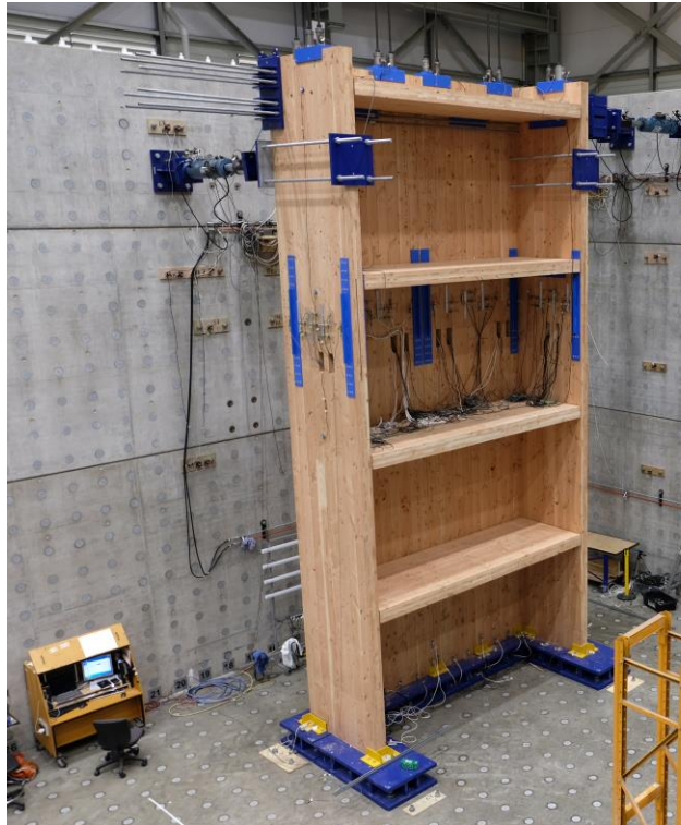
Figure 20: Core-wall test overall view
