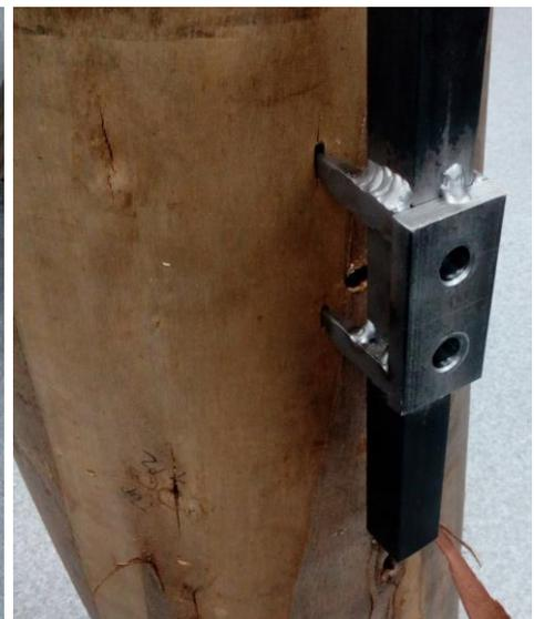
**Fig 5.** Drill stencil in position
