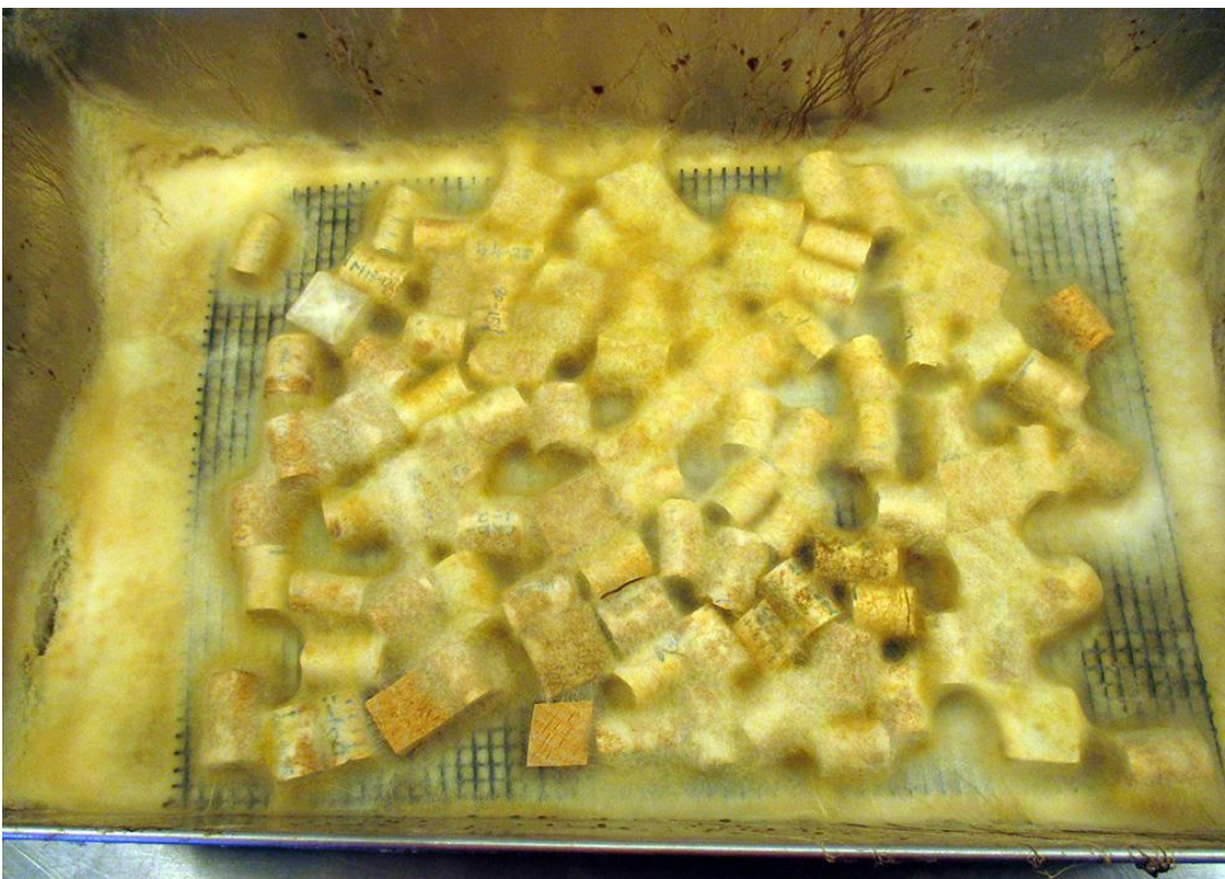
Figure 4 Brown-rot ( C. olivacea ) tray 2 after 12 week incubation period, showing extensive growth over test specimens
