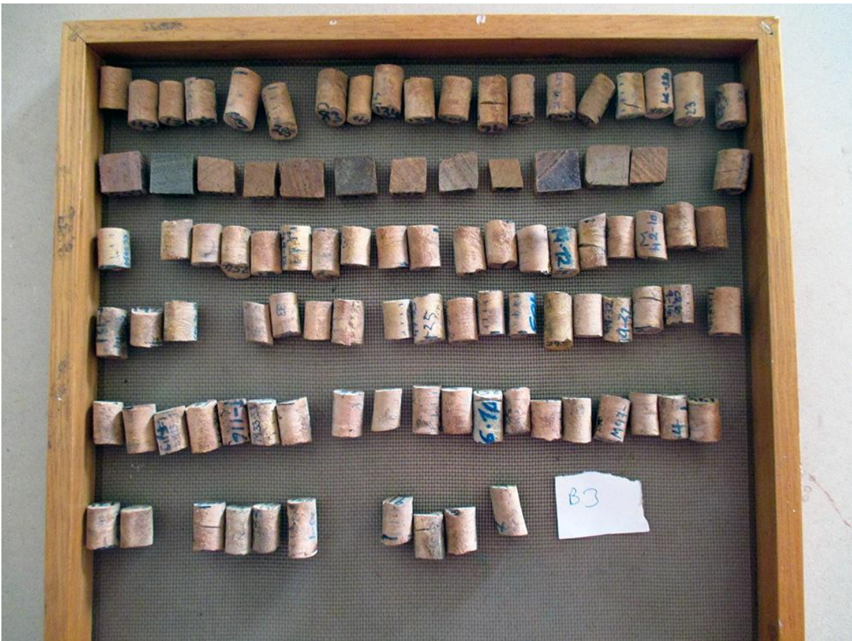
Figure 6 Cleaned and reconditioned test specimens after exposure to C. olivacea . Note shrinkage in some of the sawn test blocks.
