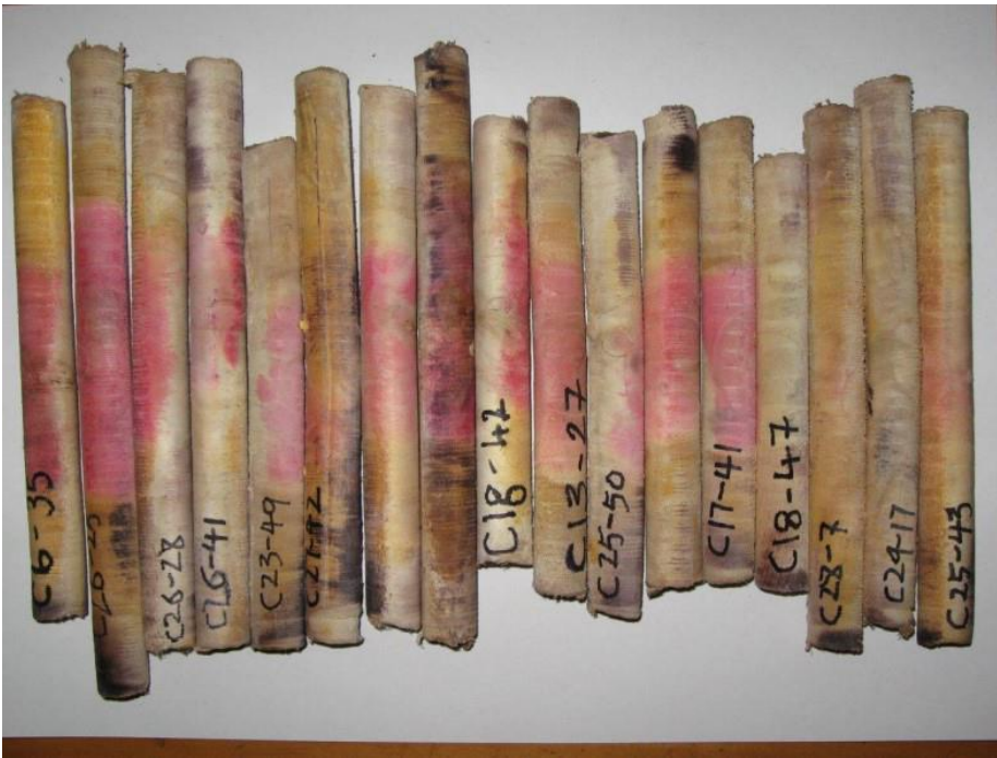
Figure 1 E. bosistoana cores stained with methyl orange. Heartwood is highlighted pink.
