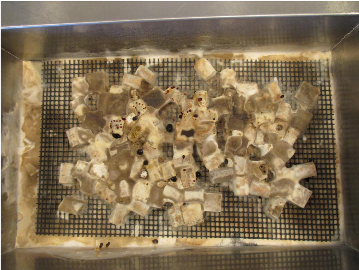
Figure 5 White-rot ( P. tephropora ) tray 2 after 12 week incubation period, showing extensive growth over test specimens.
