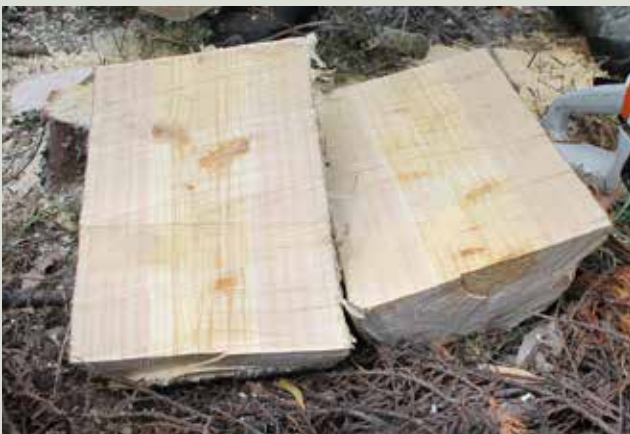
Ovens cypress log showing pruning stubs (the knotty core) and clearwood laid down outside this. The small knotty core confirms that this tree was pruned on time.
