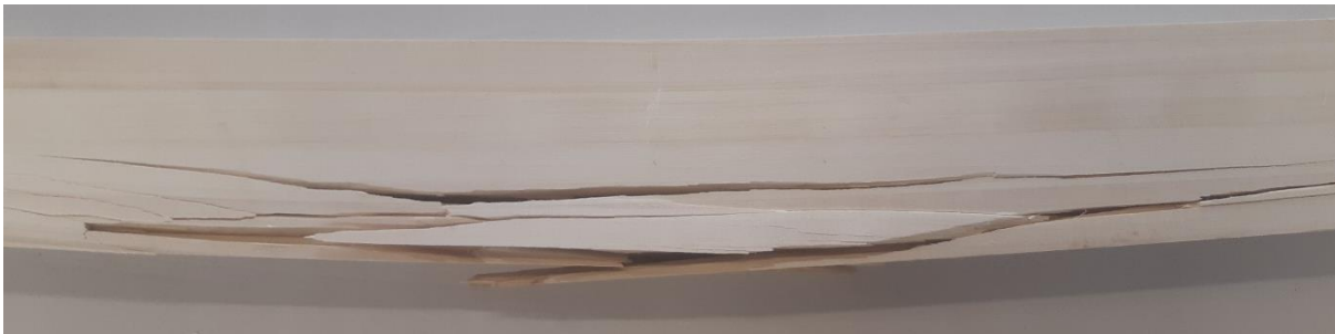
Photograph 3: Typical Tension failure in Clearwood also with compression wrinkle in Clearwood, Beam 289924
