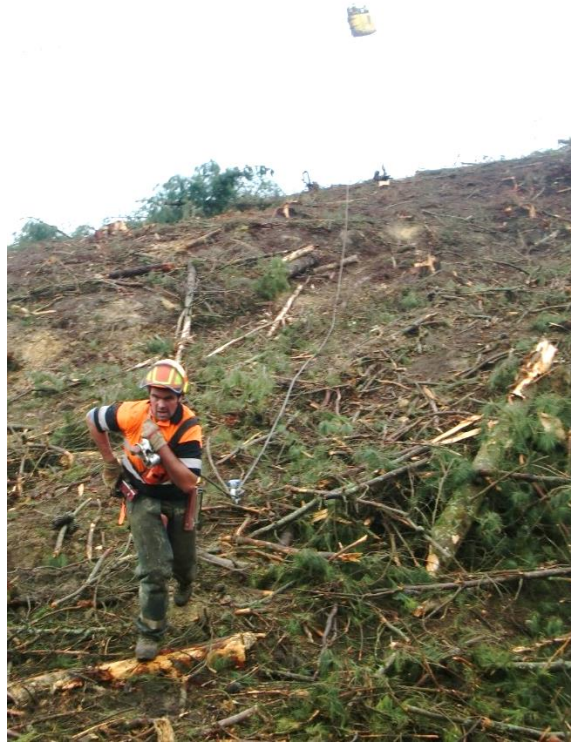
Figure 4: Setting chokers for a cable logging operation is physically very demanding work. In this scenario the choker-setter would not hook up the two larger pieces of woody debris in the photo (to the right and below his foot) as they have no economic value.
