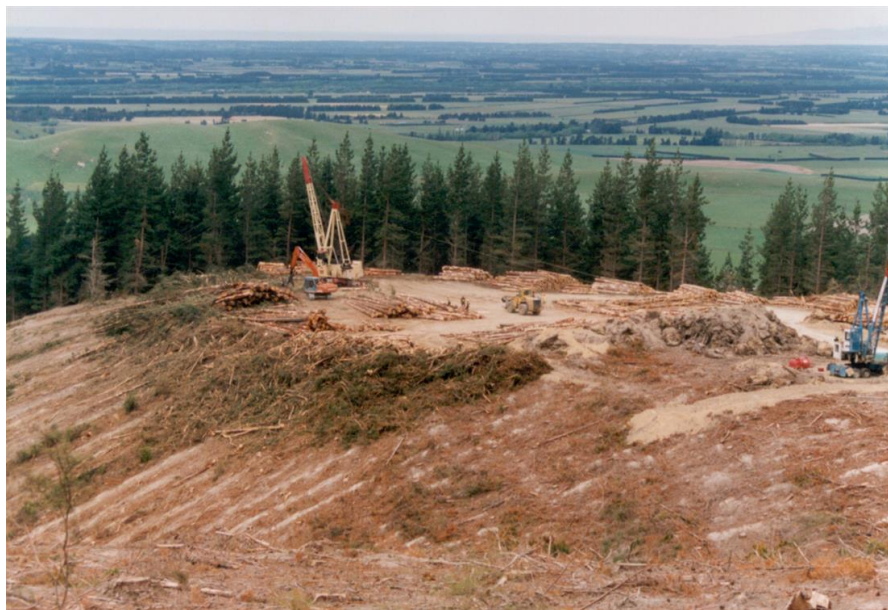
Figure 7: A typical steep terrain cable logging harvesting operation showing trees being extracted and processed into logs on the landing, whereby the harvest residue is discarded off the landing edge.
