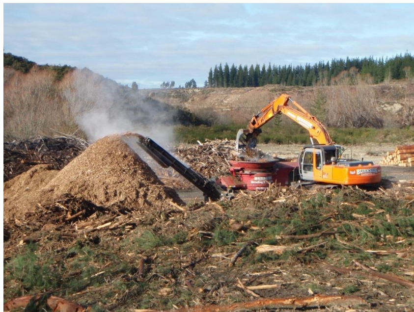
Figure 8: An excavator with a rake, combined with a tub grinder, being used to remove LWD from a super-skid. The grinder produces a hog-fuel that is used by the local mill.
