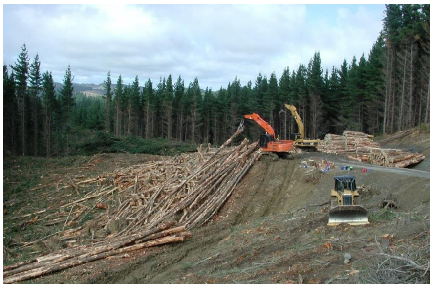
Figure 1: In this harvest operation, felled and delimbed stems are extracted to the landing for processing into logs. While the smaller harvest residues will be spread out in the cut-over, stem residues (off-cuts and slovens) from processing are discarded over the edge of the landing behind the processor.
