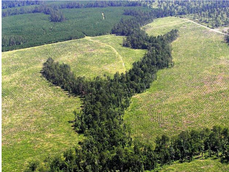
Figure 20: An aerial photo of a plantation forest (from Texas USA) showing SMZ that protects water quality. SMZ need not be no-cut zones, but enough vegetation remains to avoid direct harvesting impacts, to intercept erosion, and on steeper slopes mobilised harvest residues.
