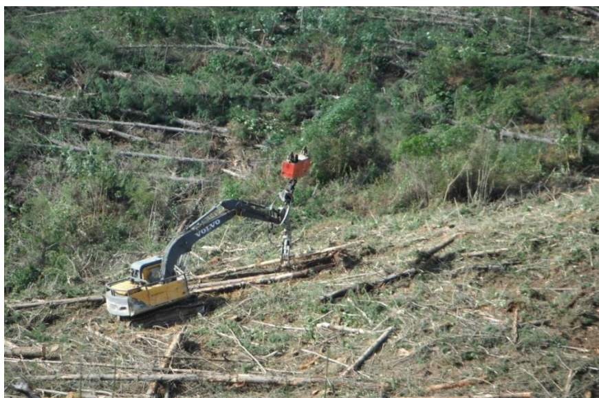
Figure 21: An excavator is used to ‘feed’ the motorised grapple extraction system. While an excavator can readily clean up the cut-over from all LWD, the risk is a greater level of soil disturbance.
