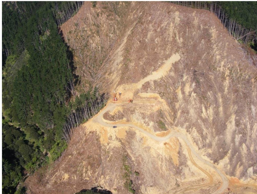
Figure 13: Aerial Photo showing extensive soil disturbance from building roads and tracks (photo: Grant Blackie)
