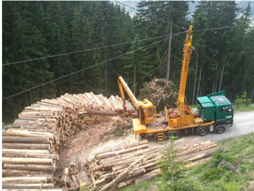
Figure 9: A European yarder system, showing the slash (just behind the yarder) being recovered and piled alongside the processed logs for subsequent grinding to make a biomass product.
