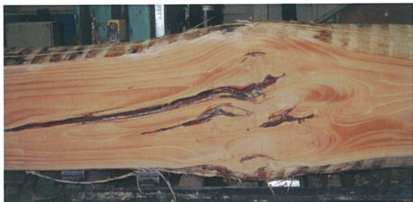
Large bark pockets associated with Nectria observed at the headrig carriage during primary breakdown.
