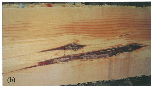
(a) Bark pocket observed during primary breakdown at the headrig. (b) The same bark pocket shown in (a) following removal of a further 25 mm flitch i.e. one board further into the log.
