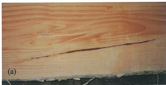
Large bark pockets associated with Nectria observed at the headrig carriage during primary breakdown.
