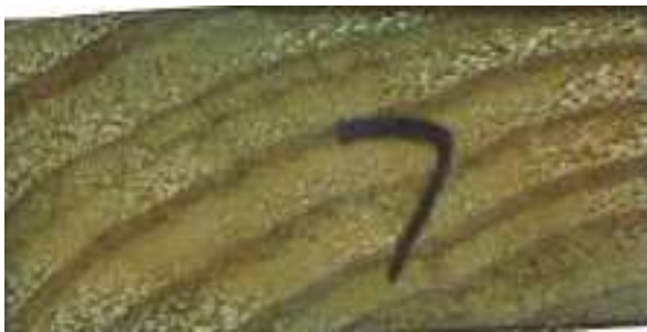
2g: Presence of 100% sapwood confirmed by sapwood/heartwood spot test
