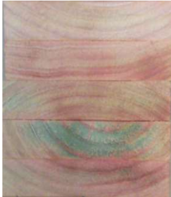
5b: The same cross-section showing the spot-test results for zinc tracer chemical with complete penetration of sapwood (pink colour). This is a Pass .
