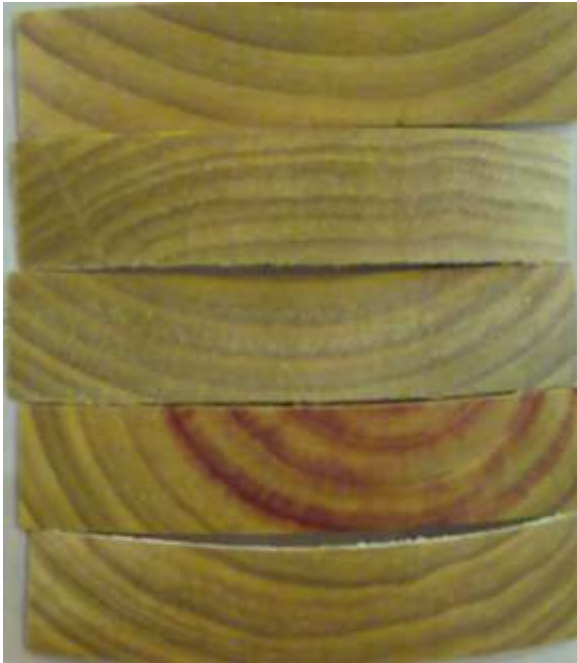
5a: The cross-section using a spot-test for sapwood/heartwood showing one sample with heartwood, which corresponds to the untreated zone in the tracer spot test showing complete penetration of sapwood, in photo on the right.
