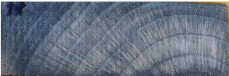
2f: Appearance of same cross-section following rubeanic acid spot-test showing complete penetration of sapwood (left of sample) and evidence of penetration in heartwood.
