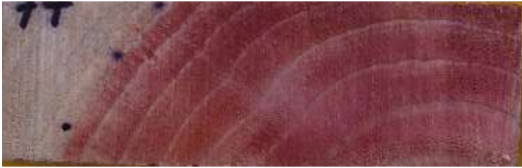
2e: Presence of sapwood and heartwood confirmed by sapwood/heartwood spot test.
