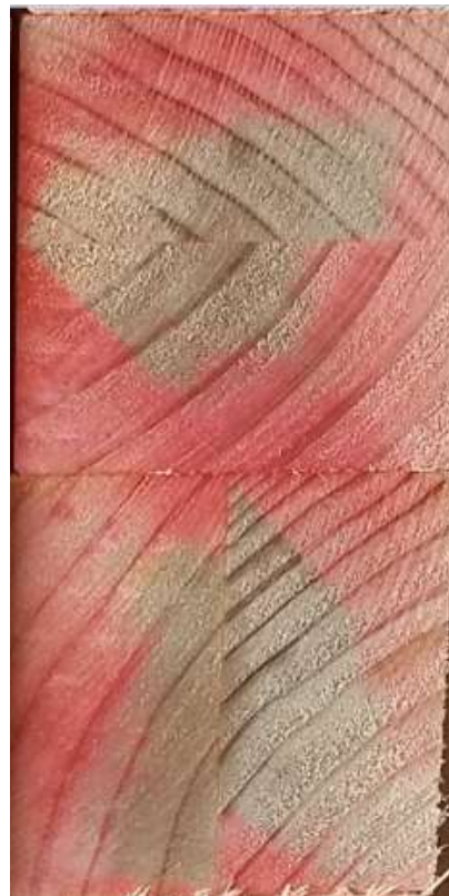
4c: The same cross-section using spot-test for sapwood/heartwood showing all sapwood that needs to be penetrated.
