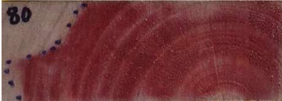
3a: Presence of sapwood and heartwood confirmed by sapwood/heartwood spot test.
