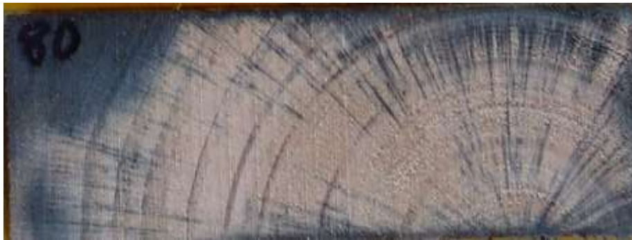
3b: The appearance of the same cross-section following the rubeanic acid spot-test showing incomplete penetration of all the sapwood (left side sample) and some evidence of penetration of heartwood. This is a penetration fail for penetration for both the sapwood and heartwood.
