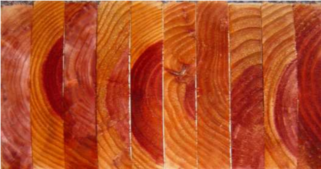
6a: Ten samples showing sapwood and heartwood confirmed by a sapwood/heartwood spot test.
