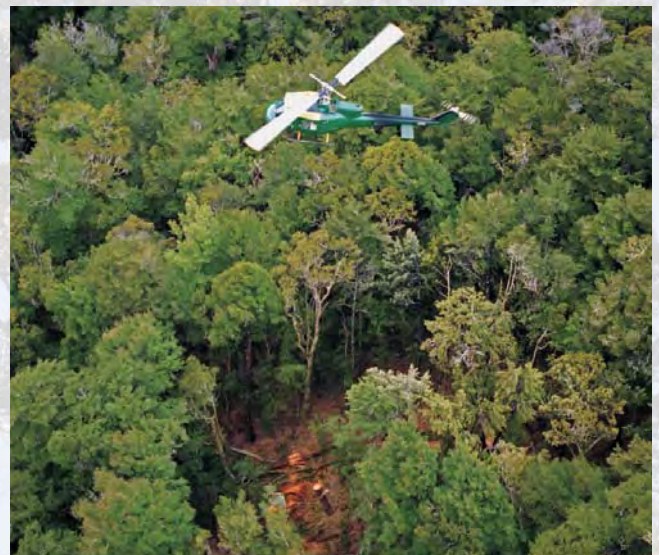
Aerial harvesting enables timber to be removed with minimal impact on the residual forest.
