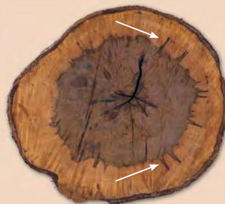
Red beech illustrating a clear delineation between the dark stained heartwood and the outer wood. The tree appears to have grown through (and healed after) a period of pinhole attack as shown by the spikes (arrow), with fungal staining at various points around the periphery of the heartwood.
