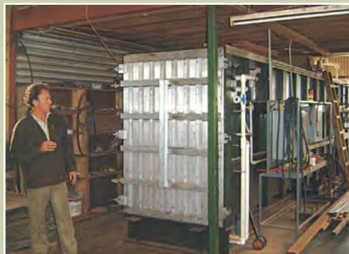
Air drying of filleted red beech (left) and the kiln used for drying (right), New Zealand Sustainable Forest Products LP sawmill, now located at Reefton.
