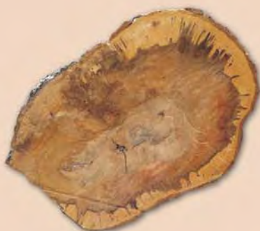
The typical black and brown lens-shaped discolouration of the wood of black beech extending longitudinally from the point of infestation and along the tunnels of Platypus beetles leading to the core of dead pathological wood.
