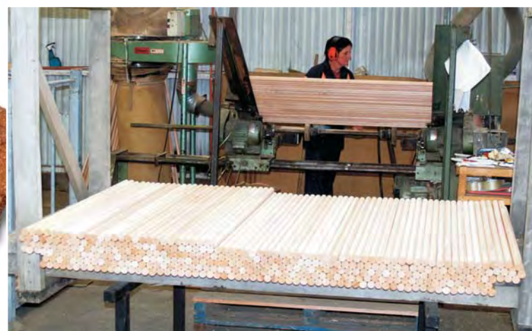
Silver beech, seen here been made into broom handles, has excellent machining properties.
