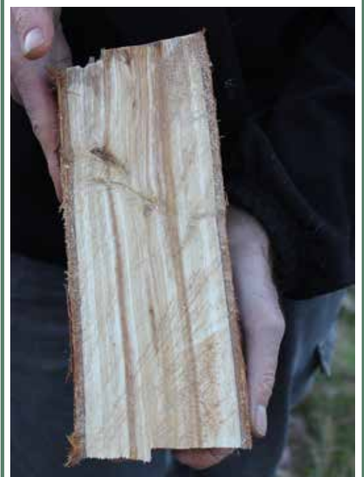
A 5-year old log showing heartwood developing and an occluded dead branch stub.
