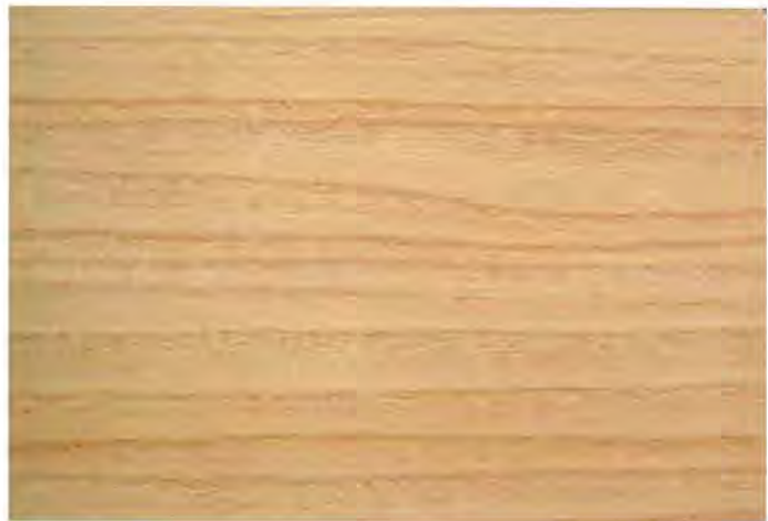
Figure 43: Veneer made from New Zealand-grown Paulownia
