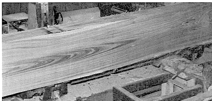
The biggest macrocarpa log in the sawing study—83% of the timber from this log was in Clears Grades.
