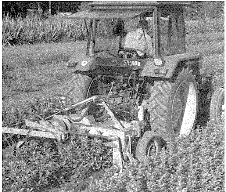
Hardwood seedlings are undercut and wrenched with tractor-mounted machinery. Conditioning encourages the formation of compact fibrous root systems.
